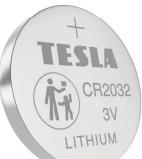
**DESCRIPTION:** Mercury Free Lithium Cell Battery, CR2032 / Non-Rechargeable **CHEMICAL SYSTEM:** Lithium Manganese Dioxide SHELF LIFE: 7 years **NOMINAL VOLTAGE:** 3 Volts **NOMINAL DIMENSIONS:** Ø 20 mm × 3.2 mm **APPLICATIONS:** Suitable for flashlights, car keys, watches, scanners etc. **STORAGE TEMPERATURE:** +10 °C to + 25 °C Should be stored in dry and cool place. **NOMINAL WEIGHT:** 3 g
